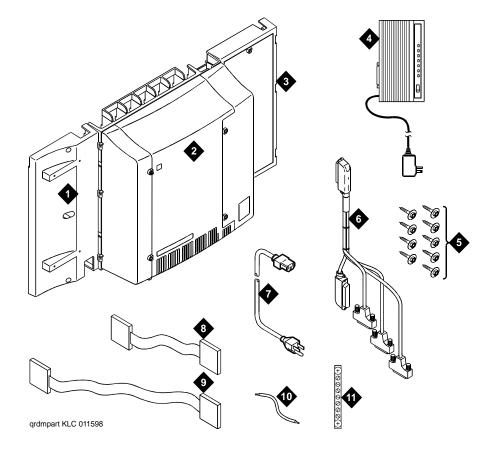
Figure 1: Equipment Packed with the Compact Modular Cabinet
